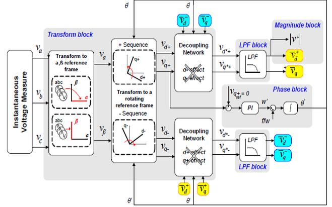
Fig.2. A diagram showing DDSRF PLL
