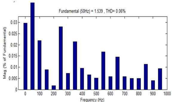
Fig.11. Total harmonic distortion of System with PLLs
