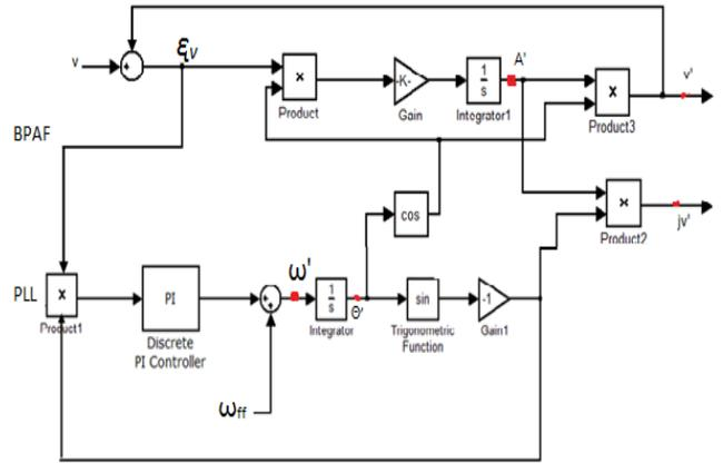
Fig.6. Quadrature Signal Generator based on an Enhanced Phase-Locked Loop structure
