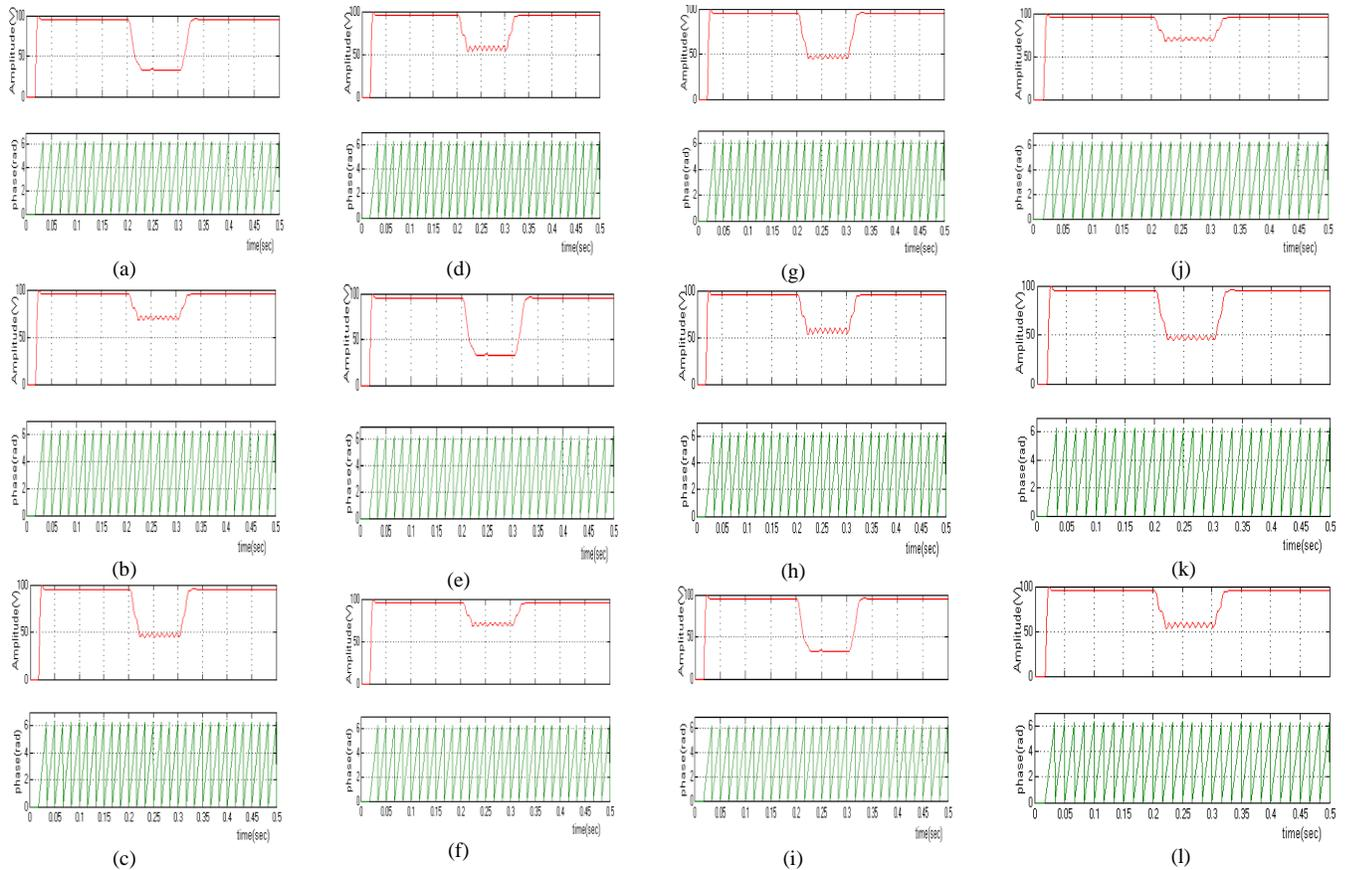
Fig.8. Magnitude and angle evaluation of the three tested PLL's in instant of four kinds of sags. (a) – (d) Magnitude (V) and angle (rad) recognition for the DDSRF PLL; (e) – (h) Magnitude (V) and angle (rad) recognition for the DSOGI PLL; (i) – (l) magnitude (V) and angle (rad) recognition for the 3phEPLL PLL
