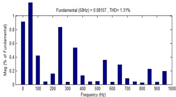
Fig.10. Total harmonic distortion of System without PLLs
