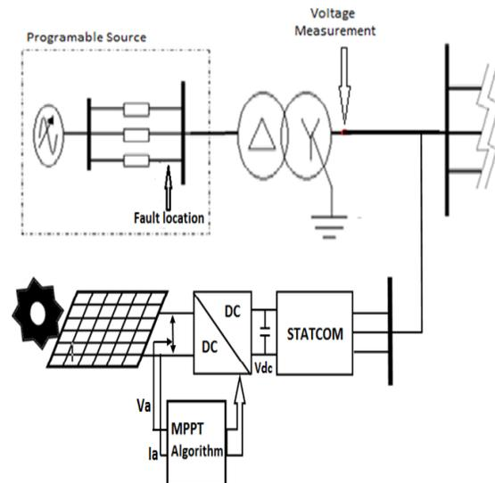
Fig.1. The proposed battery through STATCOM based synchronization techniques - Charging station connected from Photovoltaic Array
