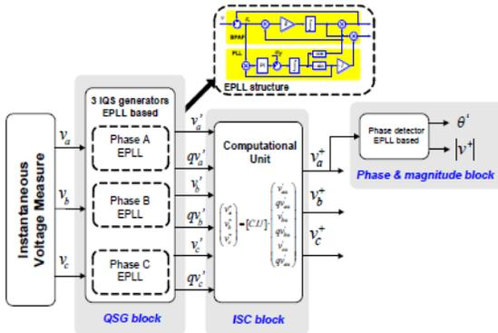
Fig.5. A diagram showing Three Phase Enhanced PLL
