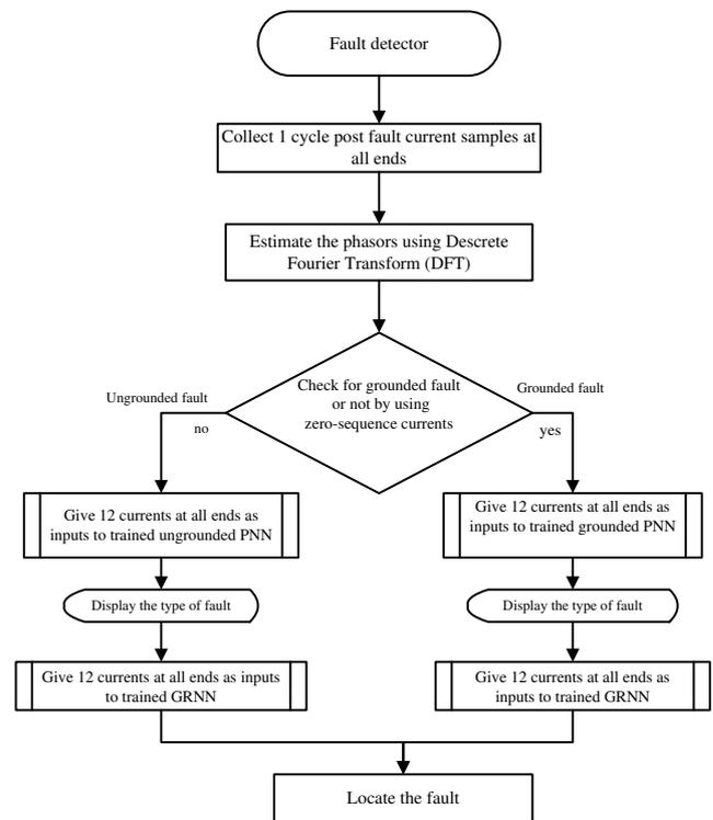
Fig.5. Flow chart for fault location in double circuit transmission line
