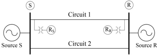
Fig. 6. Double circuit transmission network
