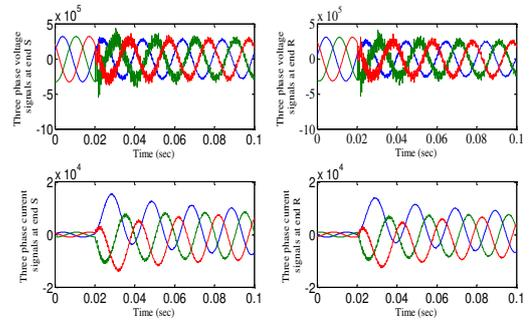
Fig. 8. Three phase voltage and current signals measured at both ends for ABC fault at 100 kms and fault inception time at 0.02 sec
