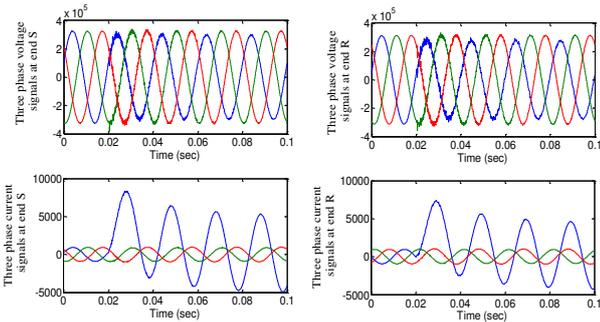
Fig.7. Three phase voltage and current signals measured at two ends for AG fault at 100 kms and fault inception time at 0.02 sec
